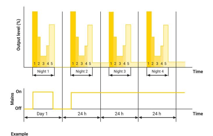
**Example:** Client needs to turn on and off for 1 Day (If possible 3 consecutive days) to set the operation time and Midpoint. And the dimming scene which was set at the factory will take place automatically the next day with this calibration.
