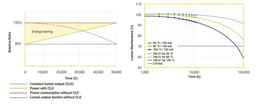
To achieve a constant light output of the module, the LED driver stores the operating hours of the LED module, powers the LED below its maximum rated lumen output, then over time increases the output current in response to the natural reduction in lumen output over the lifetime of the fitting.
